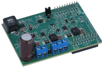
Fig.4. Inversor Texas Instruments BOOSTXL-3PHGANINV [11].
